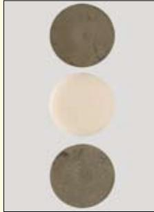
Fig. 2: Blasted Titanium surface (left), blasted Zirconium dioxide surface (middle) and etched/blasted Titanium specimen (right) all 1 cm diameter
